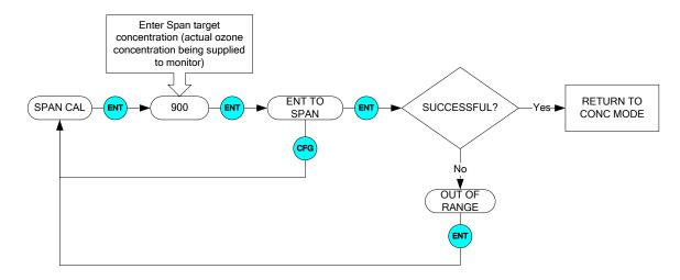
Figure 7-4: Span Cal Menu
